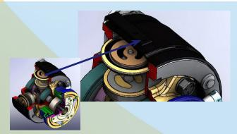
NAPA® TEMP UNIT NAPA® Temp employs a more durable piston yoke design with a wrap around discharge passage, allowing for larger volume (188cc).
